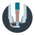
8 Solid Copper Core Center Electrode deeply inserted in the center electrode for improved thermal conductivity
