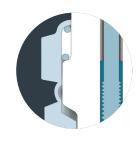
7 Triple Sealing Technology airtight seal holds compression under heavy combustion
